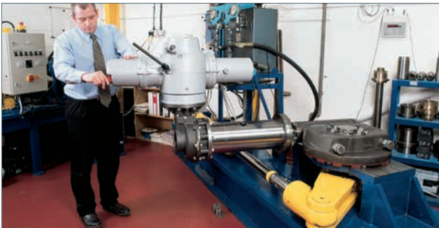
Endurance testing of prototype subsea gearbox.
