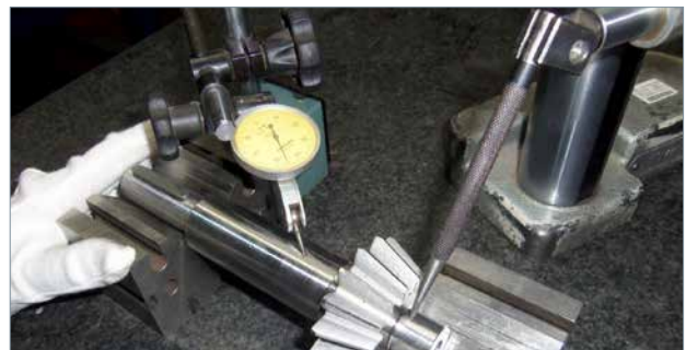
Concentricity test with dial indicator.
